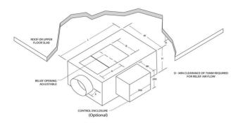
VAV terminals are suitable for Variable Air Volume supplies with options in Pneumatic, Electrical Control or Automated Control Systems (ACS) to suit most of the various applications on controls.
