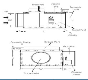
VAV systems are usually designed with diversity factor which means that the main air handler design airflow is less than the sum of the total airflow of all the VAV. This is a common design because not all of the VAV in a building will be in full load during standard operation. The unit ranges are suitable for either bypass or temperature dependent applications with a capability of handling induct pressure up to 750Pa.
